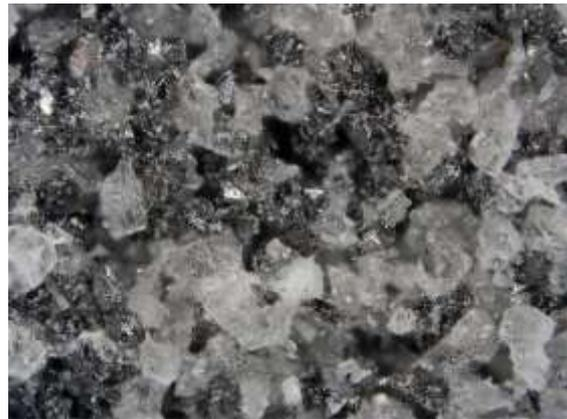
Figure 6 CBN finishing stone structure
